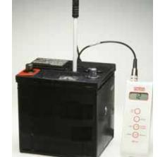
**Figure 5.7** The sulfuric acid in this battery has a pH of 1.2, which means it is extremely corrosive.
