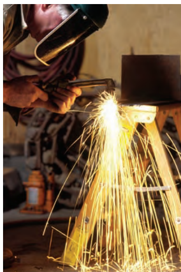
Figure 6.8 Acetylene is a gas used for welding because of the high-temperature flame produced when it is burned with oxygen. Welding with oxyacetylene produces carbon dioxide and water.
