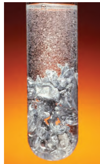
Figure 6.7B Zinc metal reacts with hydrochloric acid to produce zinc chloride and hydrogen. The bubbles shown here are hydrogen bubbles.
