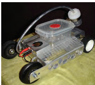
Figure 6.9 An energy source, such as a battery or photocell, can be used to produce hydrogen gas through a decomposition reaction:
