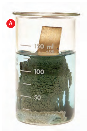
Figure 6.5A Silver crystals and a blue-green solution of copper nitrate are formed when copper metal is dipped in a solution of silver nitrate.
