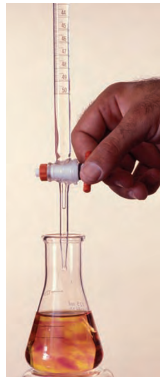
Figure 6.7A This equipment allows precise amounts of an acid to be added to a base.
