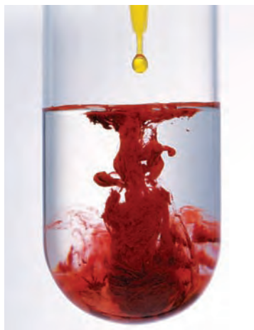
Figure 6.6A When potassium chromate, K_2CrO_4 , is added to silver nitrate, AgNO_3 , the precipitate formed is silver chromate, Ag_2CrO_4 .
