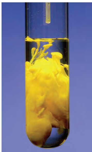
Figure 6.6B Yellow lead(II) iodide was used in the 18th century as a pigment in paints. Due to its toxicity, it is no longer used in paints.
